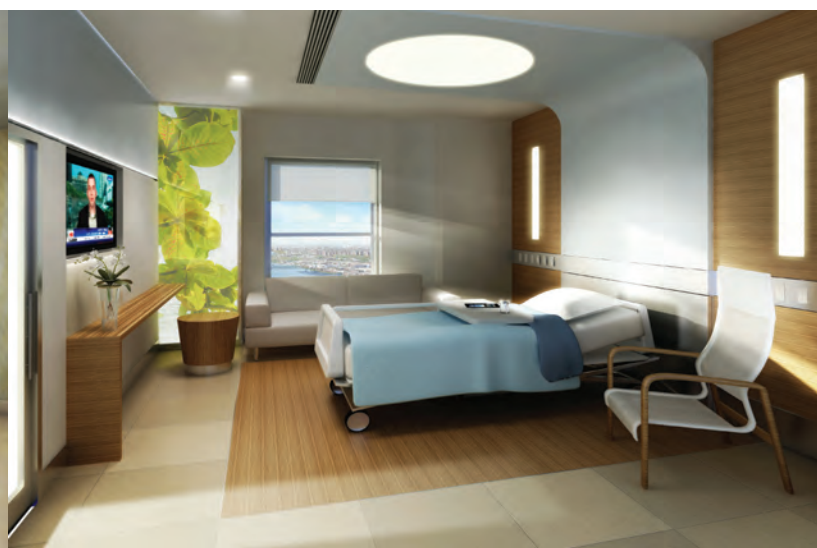
Figure 4. Programmed LED settings replicate the circadian rhythms of rise, awake, and decompress for sleep. In Pediatrics, accent wall color can be illuminated in the patient's preference without a paint change.
